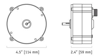
Our model RT9CN communicates rotational position feedback to your PLC via the CANbus SAE J1939 interface. The heart of this sensor is a precision plastic-hybrid position potentiometer which provides a "absolute" position and does not ever have to be reset to a "home" position after a power loss or planned shutdown.
