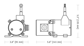
The PT8510 can operate from an unregulated 14.5 to 40 VDC power supply while providing an output signal that is proportional to the linear movement of it's measuring cable. The PT8510 has a maximum measurement range up to 60" and has 4 output signal options to choose from: 0...10, 0...5, -10...+10 and -5...+5 Vdc.
