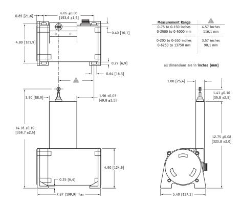
Note: Dimensions not valid for "increased cable tension" option. Consult factory for dimensions.
